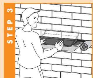
First tray is then inserted into position, bedded on mortar. Two bricks are then mortar bedded and wedged in position in the tray. A caviweep is fitted in the centre perp.
