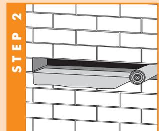
A flashing turned 25mm into the wall is bedded on mortar.
